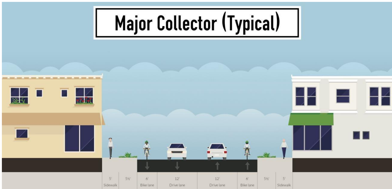
Figure 17: Typical Major Collector
