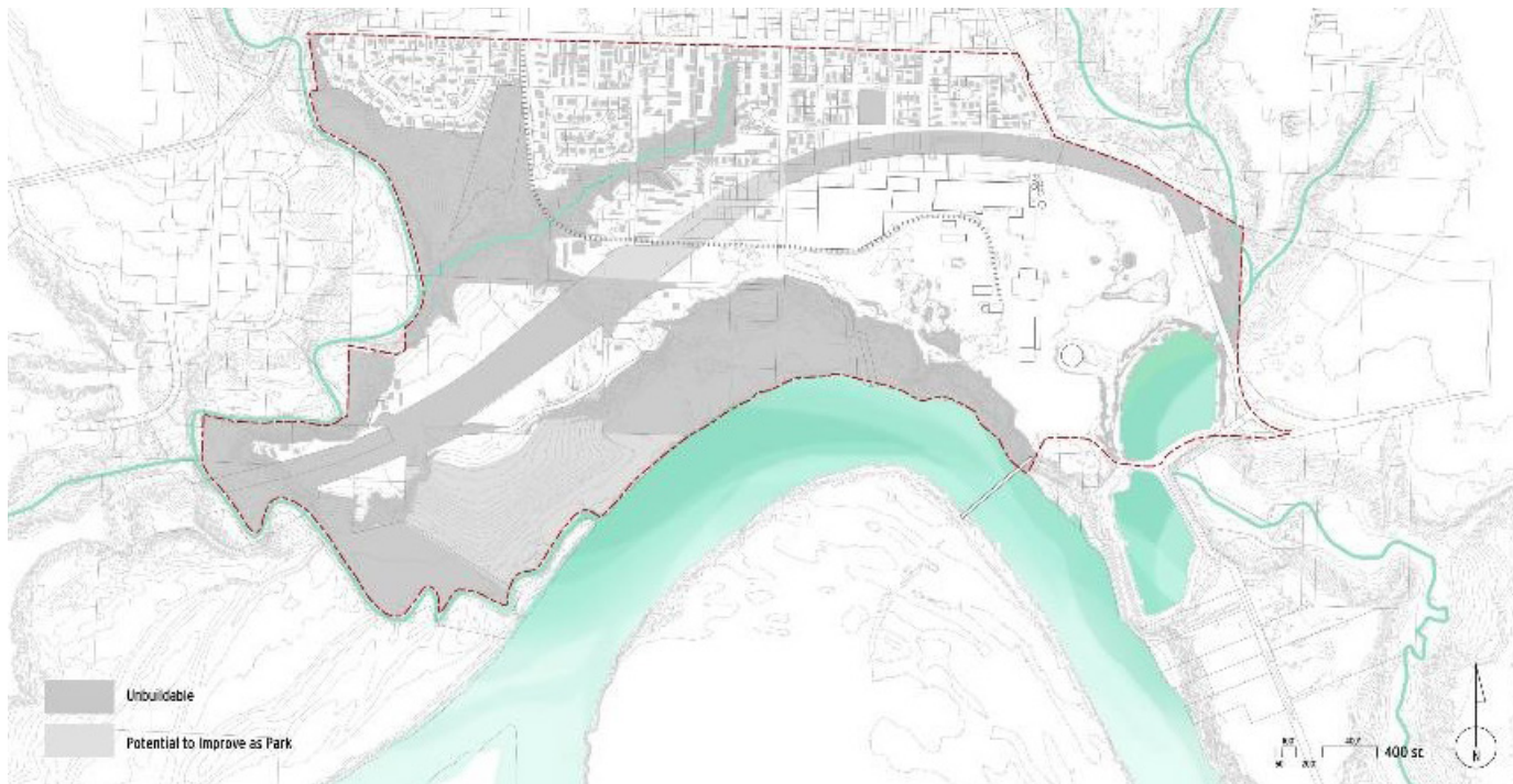
FIGURE 2. DIAGRAM OF UNBUILDABLE LAND IN THE RIVERFRONT AREA (INCLUDES STEEP SLOPES, FLOODPLAIN, BYPASS, EXISTING PARKS)
