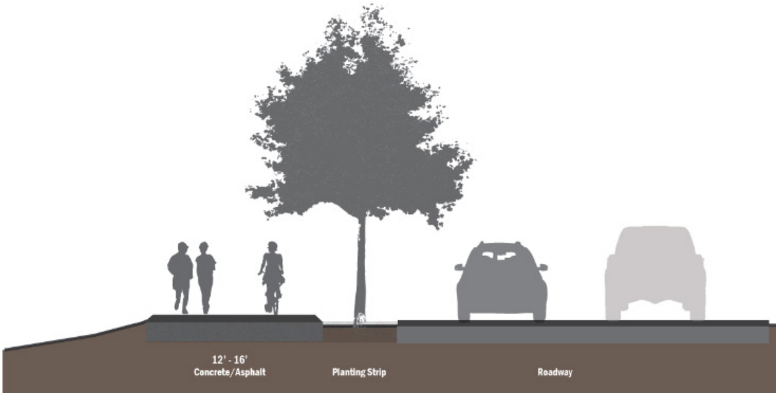
FIGURE 28. URBAN MULTI-USE TRAIL CROSS SECTION
