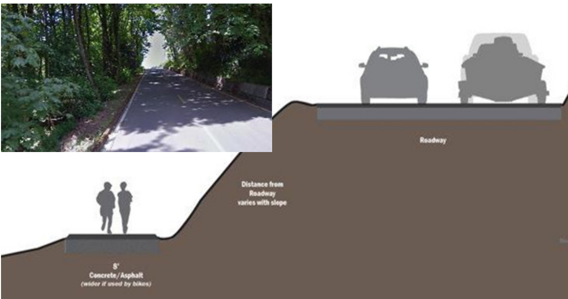
FIGURE 29. CROSS-SECTION FOR ROGER'S LANDING ROAD MULTI-USE PATH
