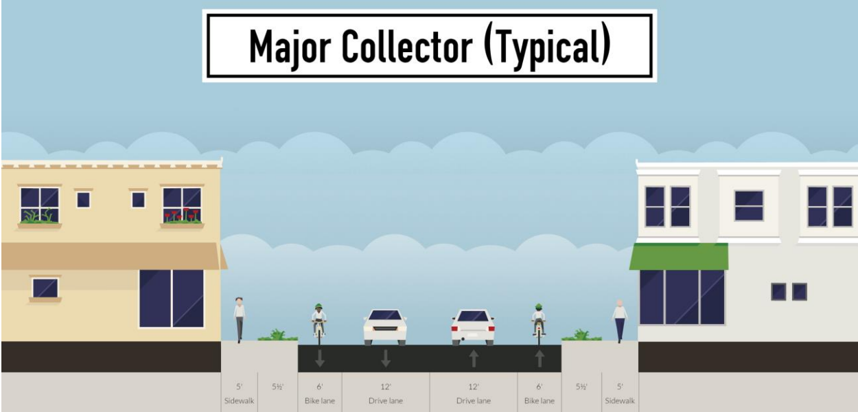
Figure 17: Typical Major Collector
