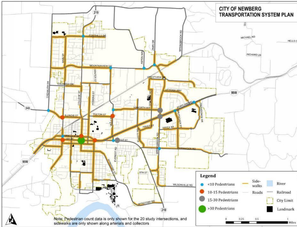
Figure 3: Pedestrian Volumes and Existing Sidewalk Network
