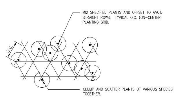
WATER QUALITY SWALE PLANT SPACING DETAIL
