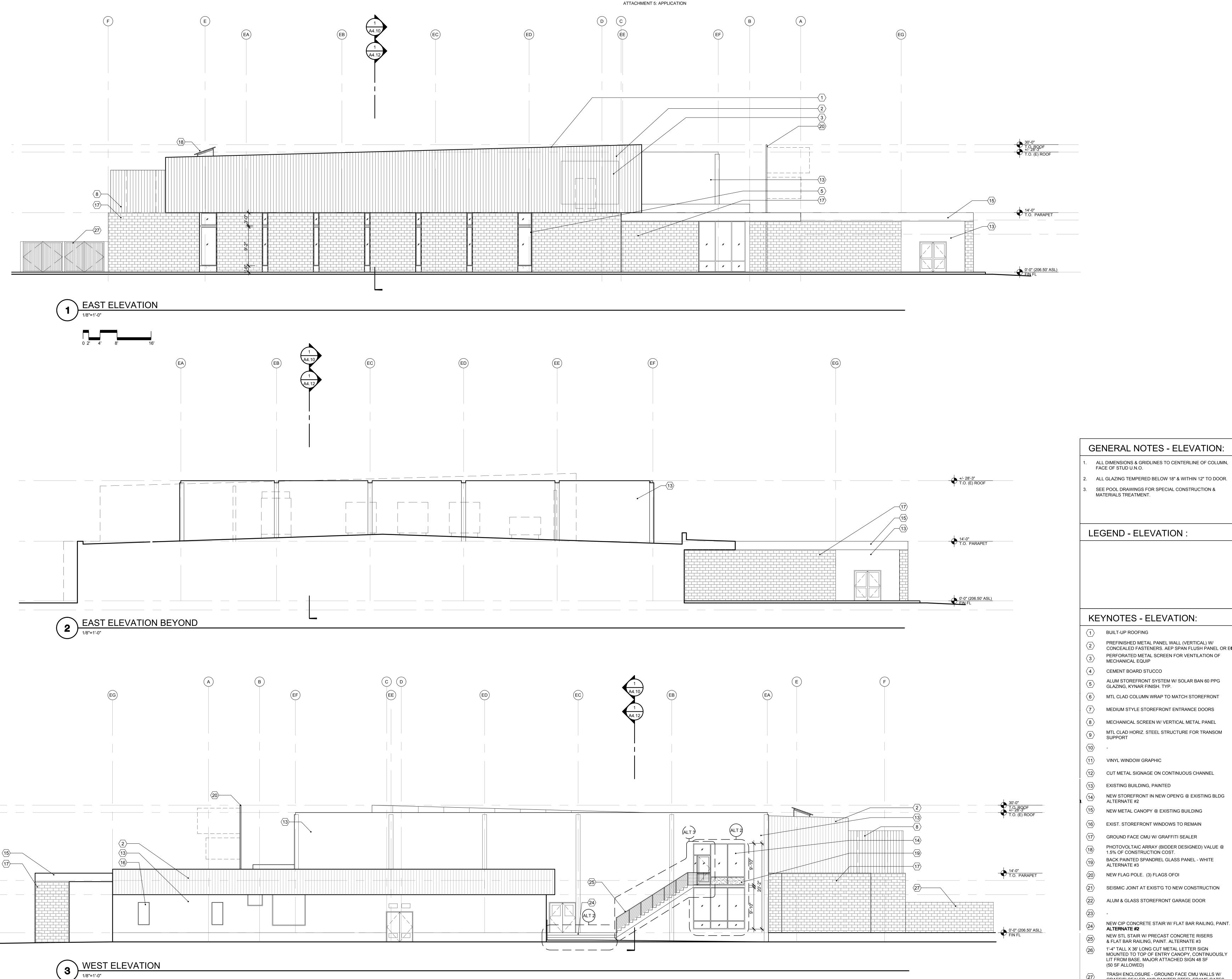
TRASH ENCLOSURE - GROUND FACE CMU WALLS W/ GRAFFITI SEALER AND PAINTED STEEL FRAME GATES **(27)** WITH VERTICAL METAL PANEL.
