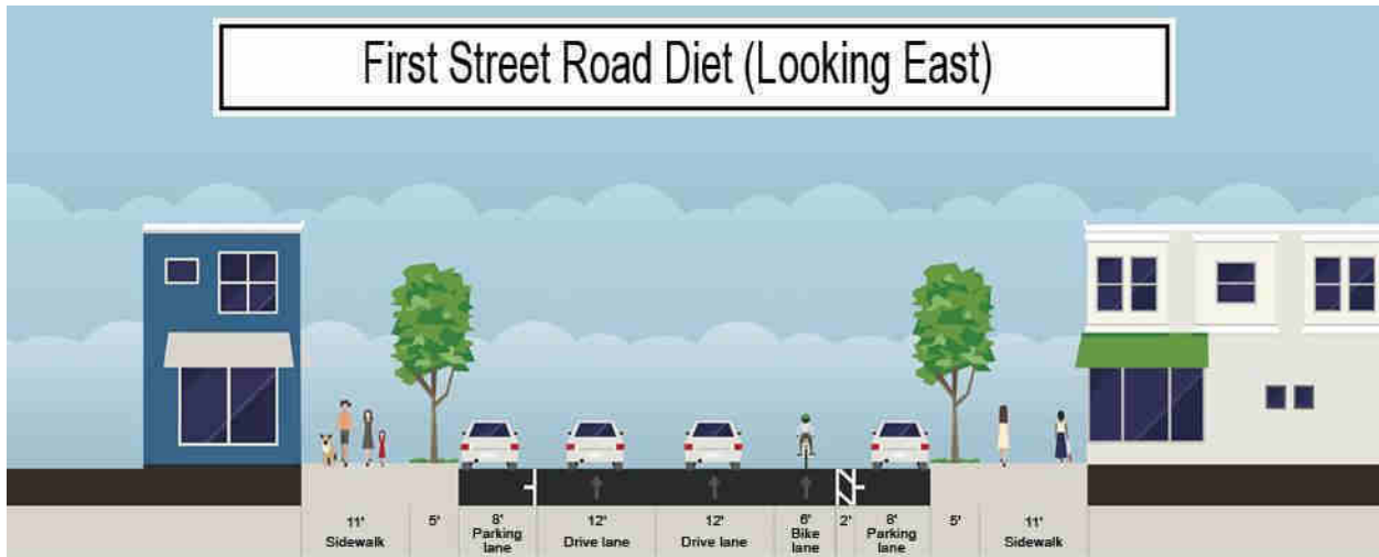
Appendix 5: First Street Permanent Work with Planter
