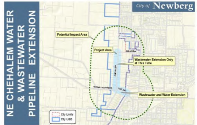
FIGURE 4 EXTENDING THE PUBLIC WASTEWATER LINE
