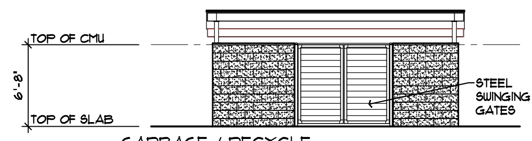
GARBAGE / RECYCLE NORTH BUILDING ELEVATION SCALE: 1/8" = 1'-0"
