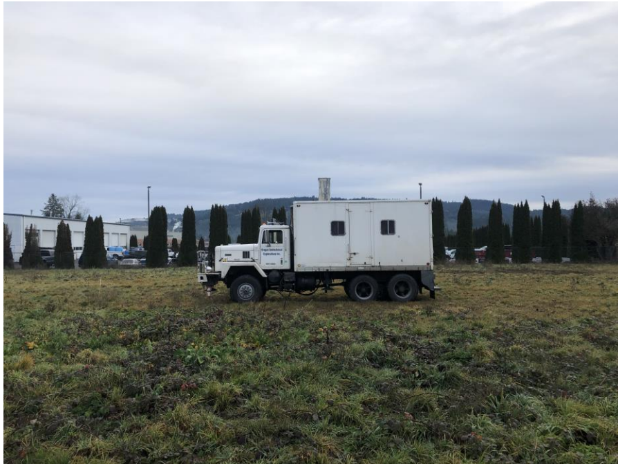
Cone Penetrometer Testing
