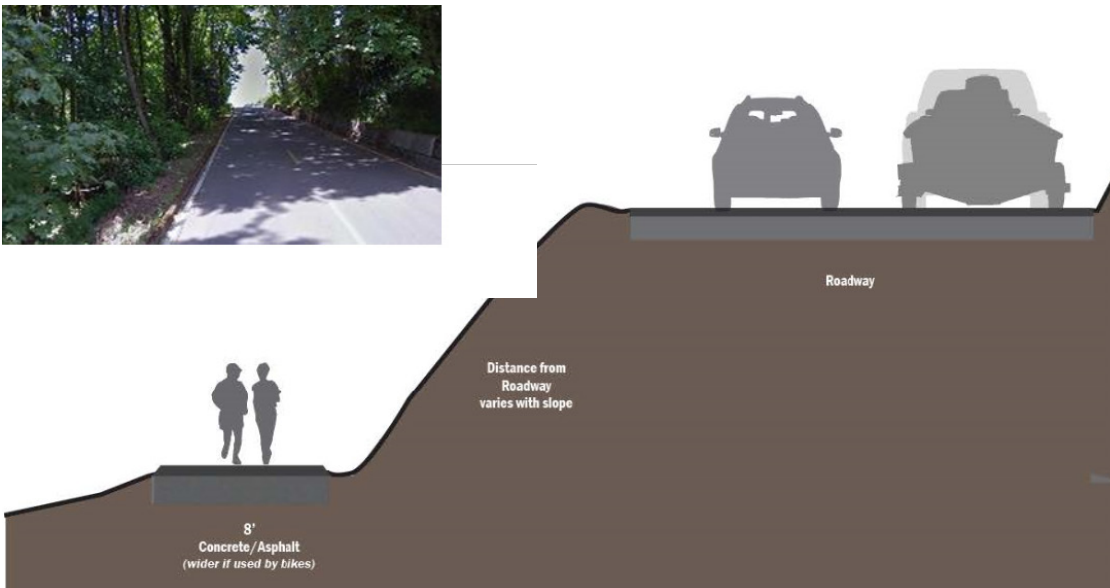
FIGURE 29. CROSS-SECTION FOR ROGER'S LANDING ROAD MULTI-USE PATH
