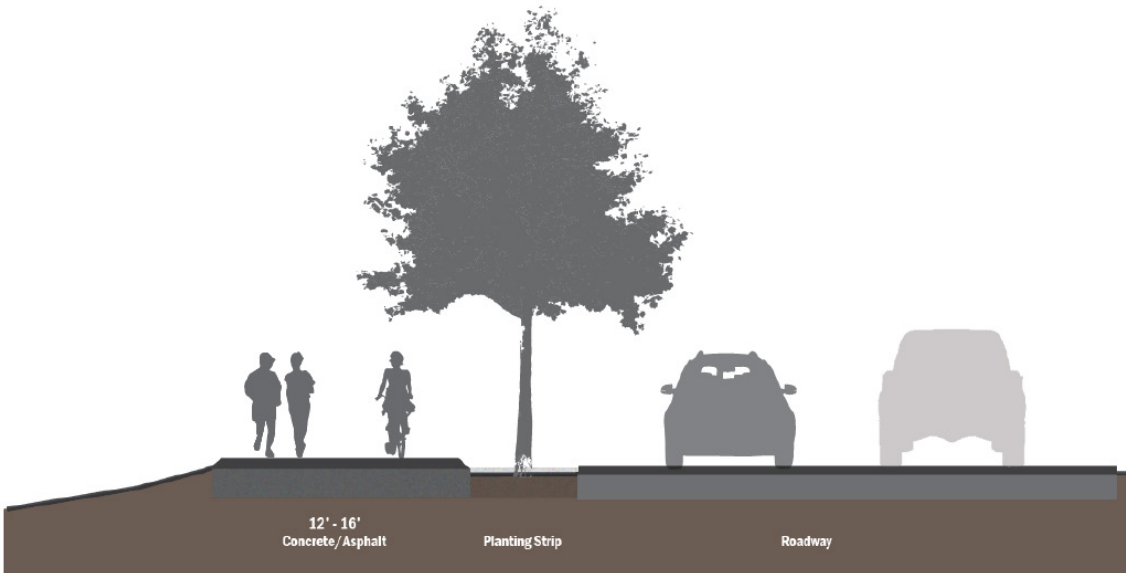
FIGURE 28. URBAN MULTI-USE TRAIL CROSS SECTION
