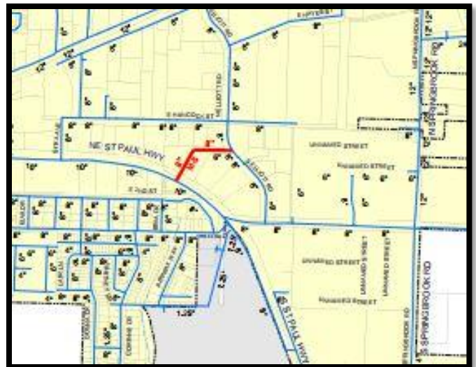
FIGURE 25 FIRE FLOW UPGRADES
