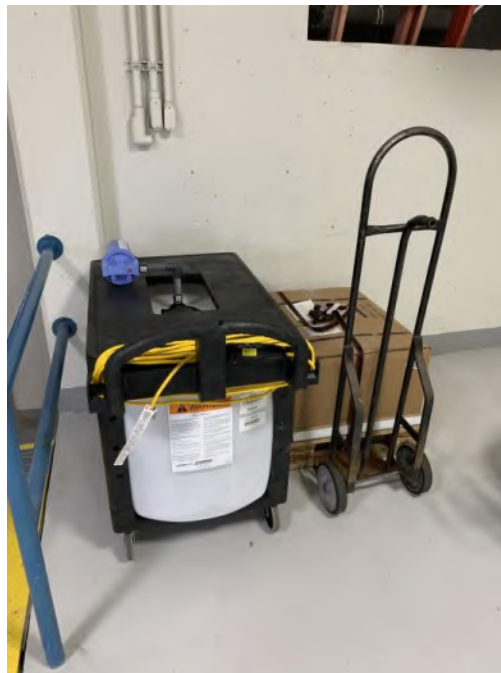
Figure 3.21 – Unrestrained Rolling Carts
