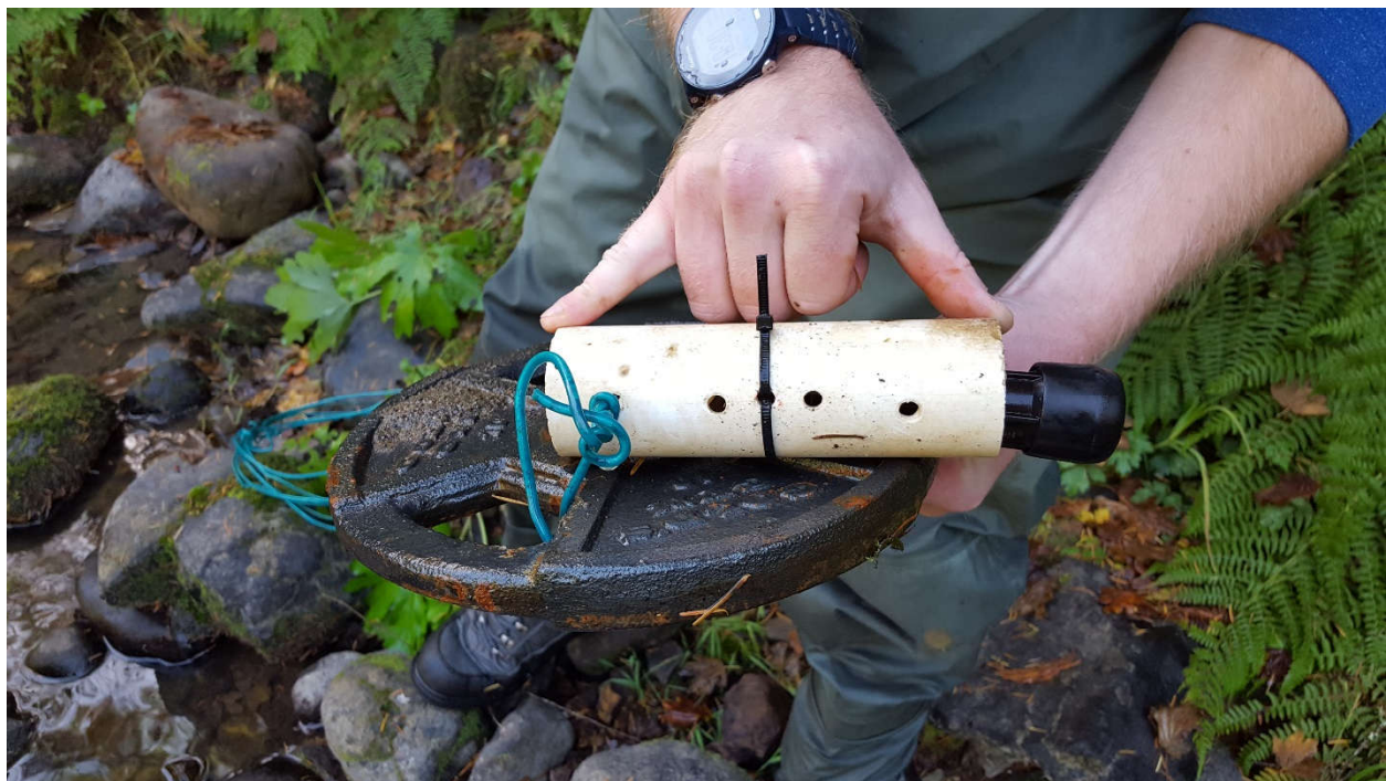
Figure 9: Weighted Plate Temperature Logger Deployment Method
