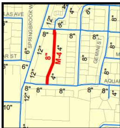
FIGURE 44 EXPANDING WATERLINE TO ELIMINATE DEFICIENT WATER FLOW AND FOR FUTURE GROWTH
