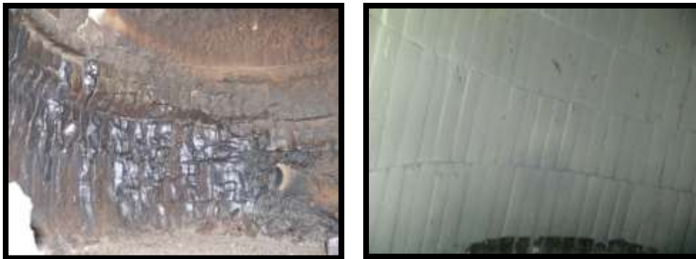
FIGURE 16 DEHYDRATION UNIT BURNER BEFORE AND AFTER CONDITION
