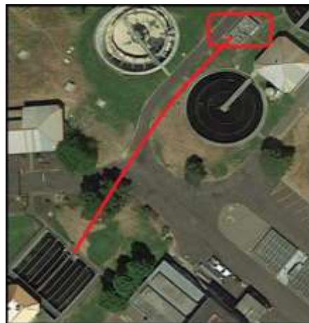
FIGURE 32 INSTALLATION OF A SECOND (PARALLEL) PIPE FROM THE CLARIFIER EFFLUENT TO THE CHLORINE CONTACT BASIN
