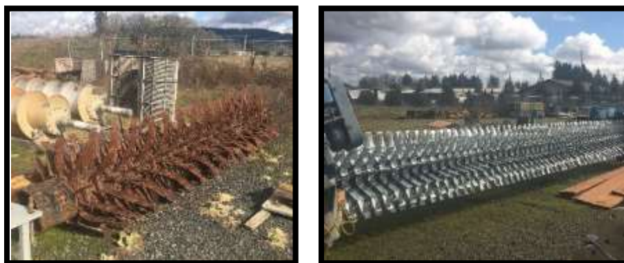
FIGURE 17 OLD ROTOR (LEFT) NEW ROTOR (RIGHT)
