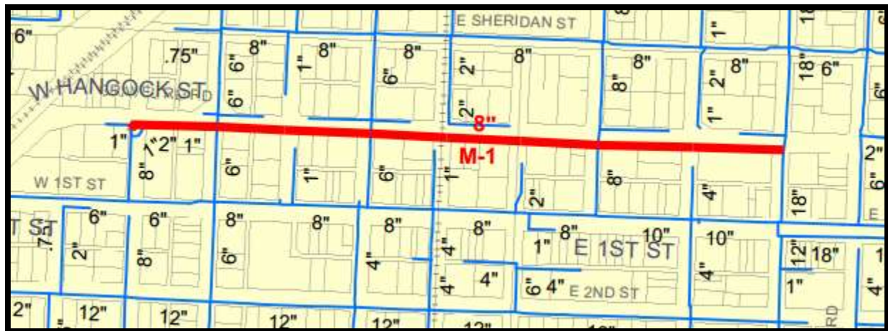
FIGURE 39 REPLACING DEFICIENT PIPE AND INADEQUATE FIRE HYDRANTS ON HANCOCK STREET
