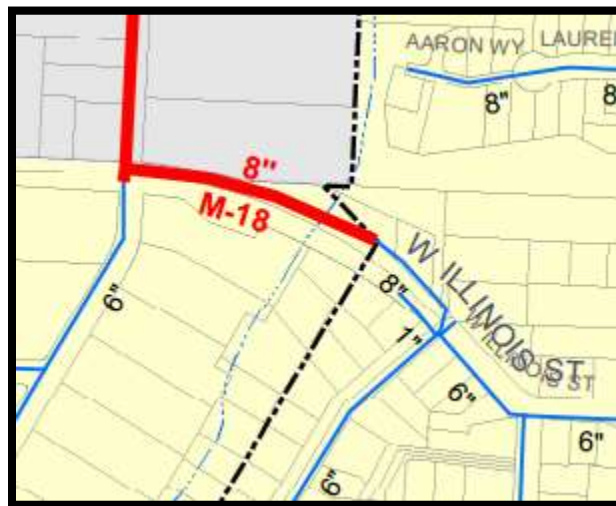
FIGURE 45 EXPANDING WATERLINE TO ELIMINATE WATER DEFICIENCY AND FOR FUTURE GROWTH
