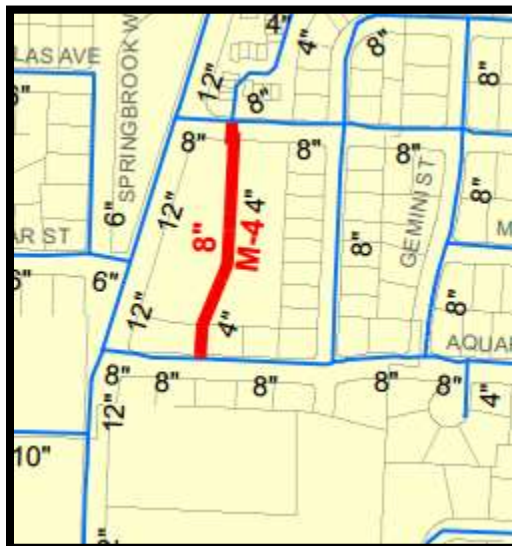
FIGURE 329 EXPANDING WATERLINE TO ELIMINATE DEFICIENT WATER FLOW AND FOR FUTURE GROWTH
