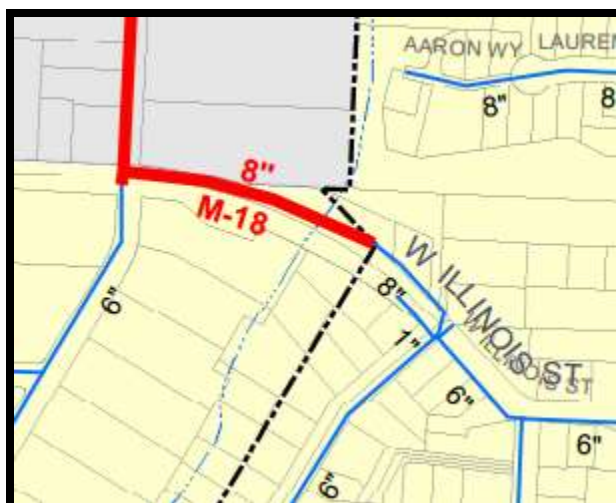
FIGURE 33 EXPANDING WATERLINE TO ELIMINATE WATER DEFICIENCY AND FOR FUTURE GROWTH
