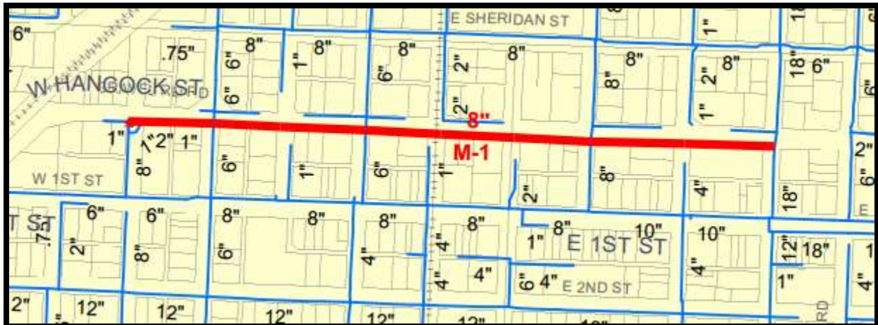
FIGURE 274 REPLACING DEFICIENT PIPE AND INADEQUATE FIRE HYDRANTS ON HANCOCK STREET
