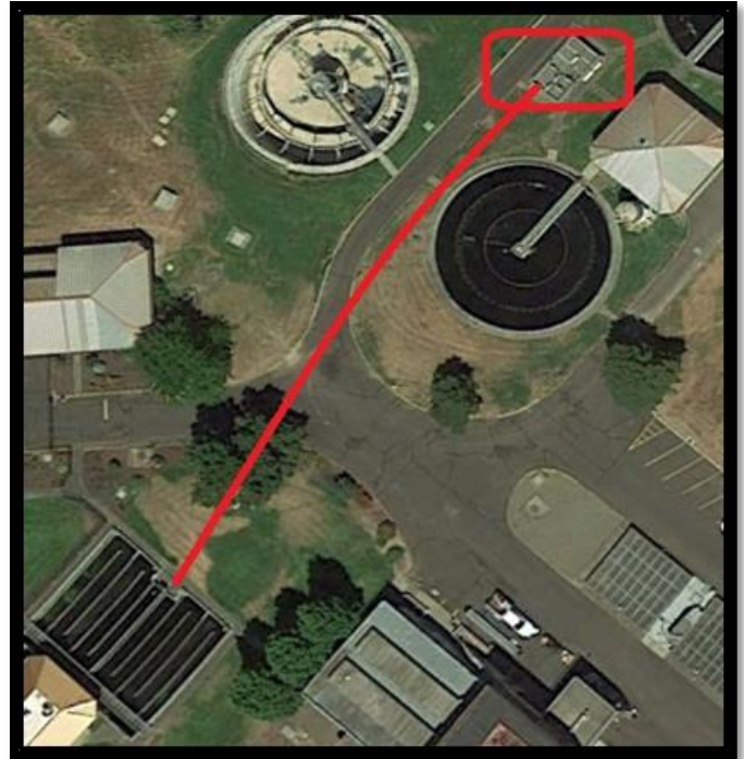
FIGURE 15 INSTALLATION OF A SECOND (PARALLEL) PIPE FROM THE CLARIFIER EFFLUENT TO THE CHLORINE CONTACT BASIN
