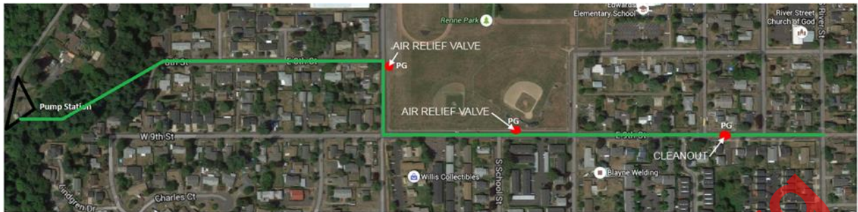
Figure 1 Force Main Alignment and Pressure Gauge Locations
