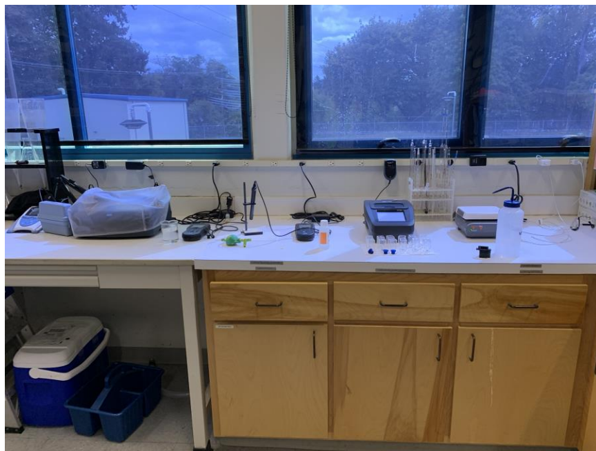
Figure 3.43 – Unrestrained Equipment on Lab Counter
