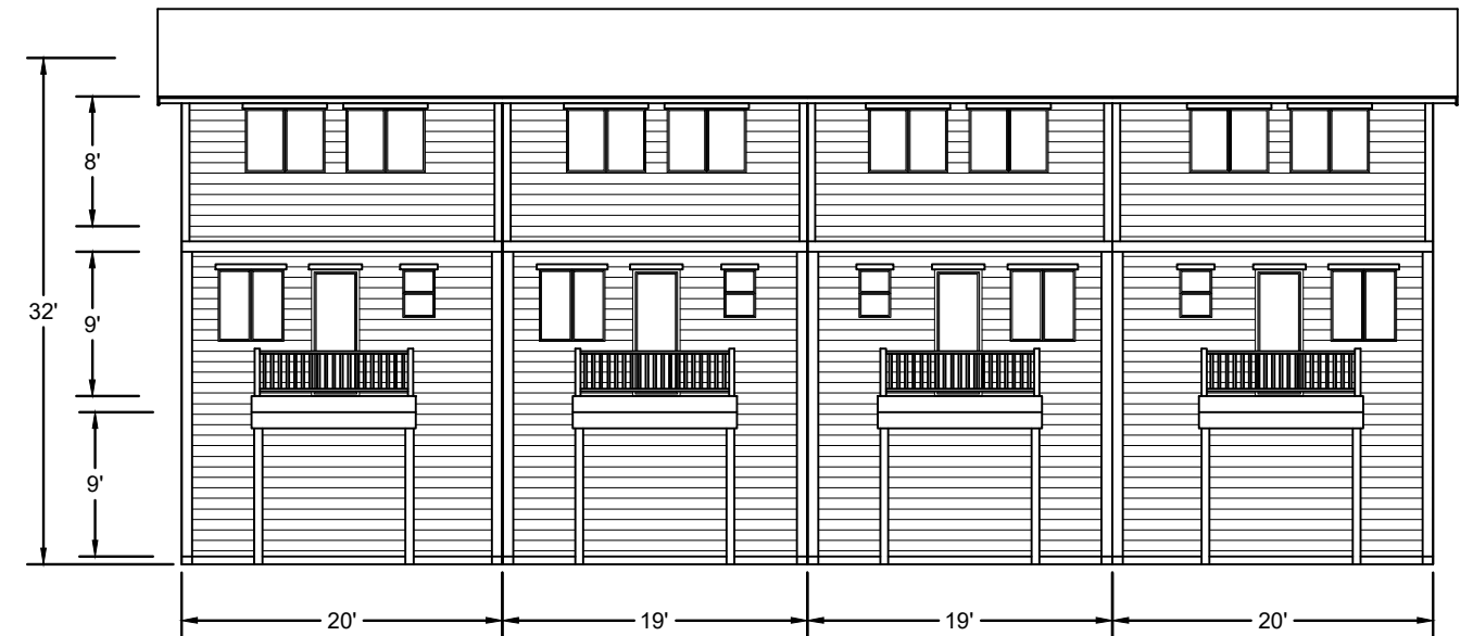
4-PLEX TOWNHOUSE - TYPICAL REAR ELEVATION
