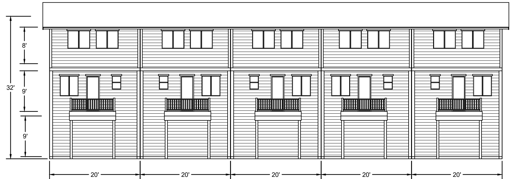
5-PLEX TOWNHOUSE - TYPICAL REAR ELEVATION
