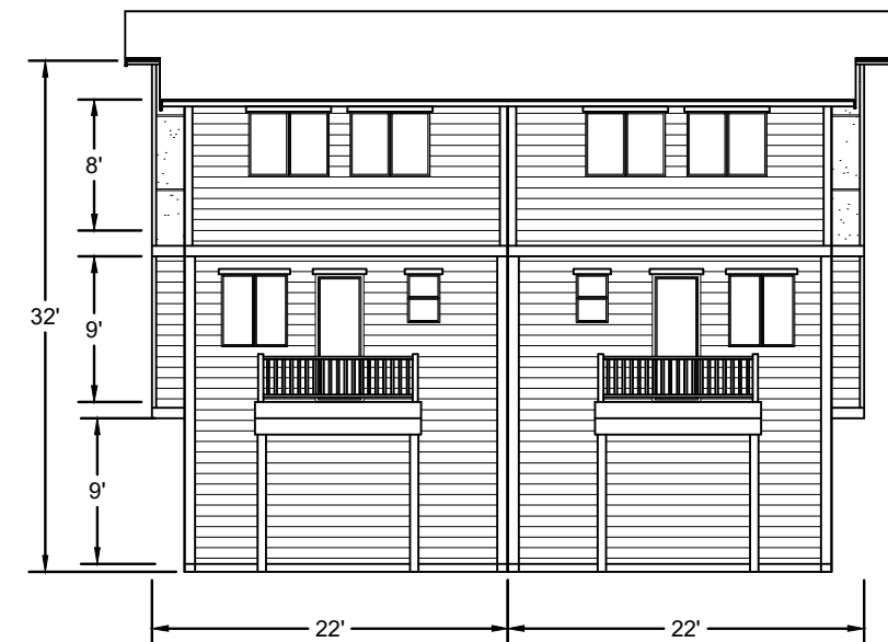
2-PLEX TOWNHOUSE - TYPICAL REAR ELEVATION
