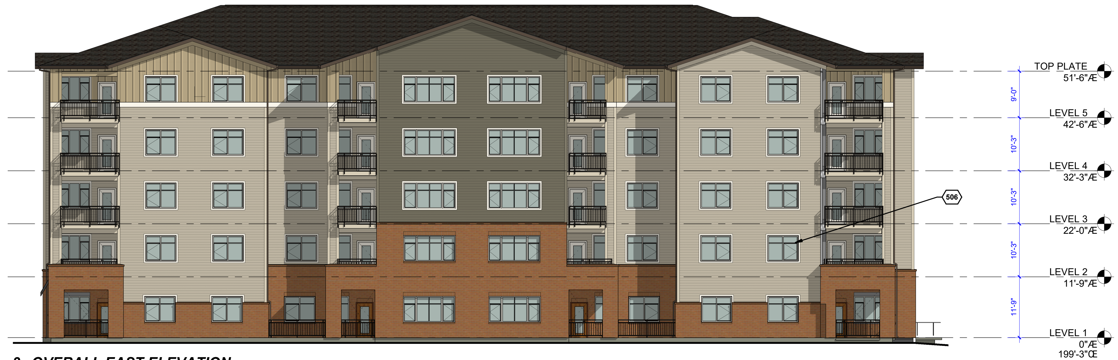
3. OVERALL EAST ELEVATION
