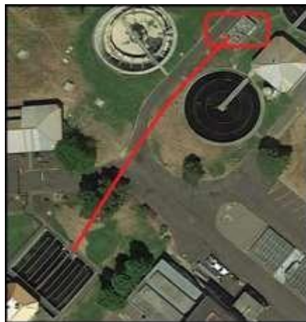
FIGURE 26 INSTALLATION OF A SECOND (PARALLEL) PIPE FROM THE CLARIFIER EFFLUENT TO THE CHLORINE CONTACT BASIN
