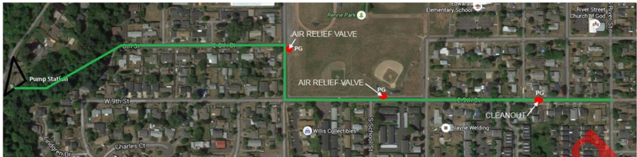
Figure 1 Force Main Alignment and Pressure Gauge Locations
