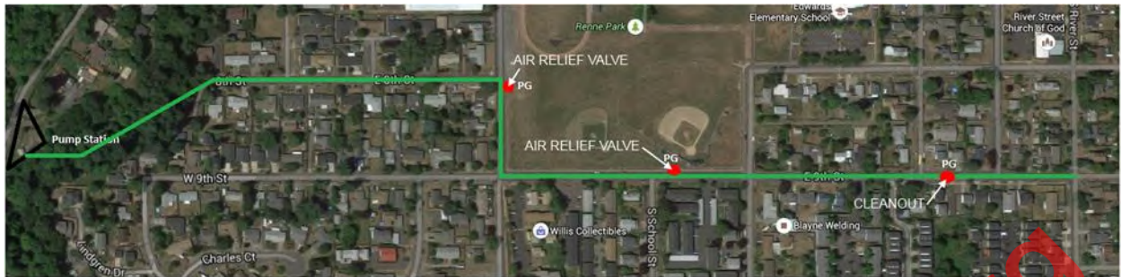
Figure 1 Force Main Alignment and Pressure Gauge Locations
