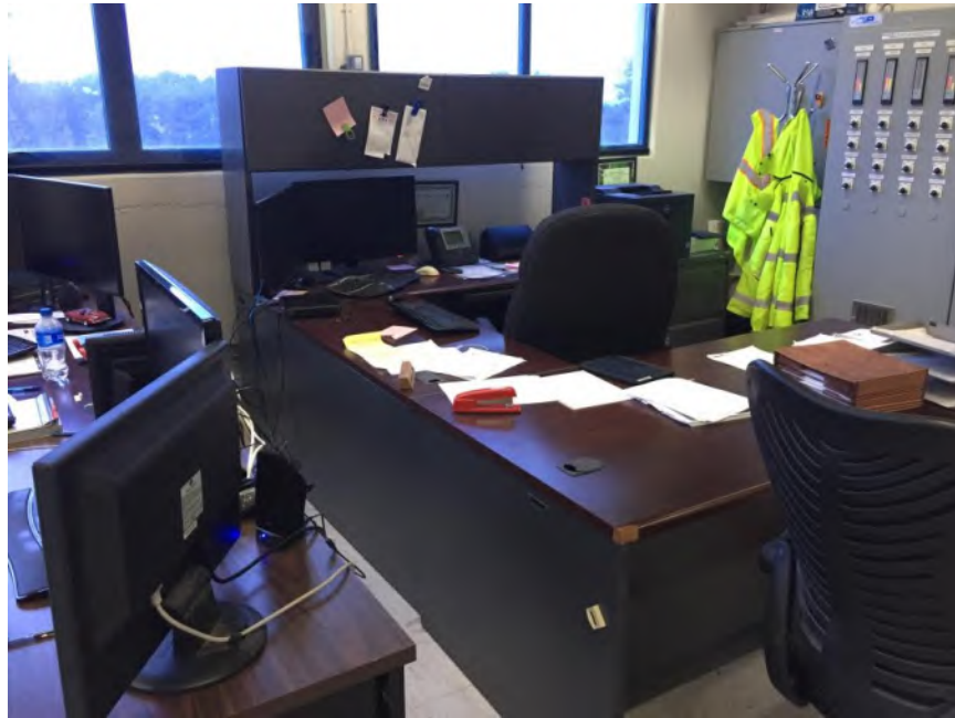
Figure 3.42 – Unrestrained Computer Equipment
