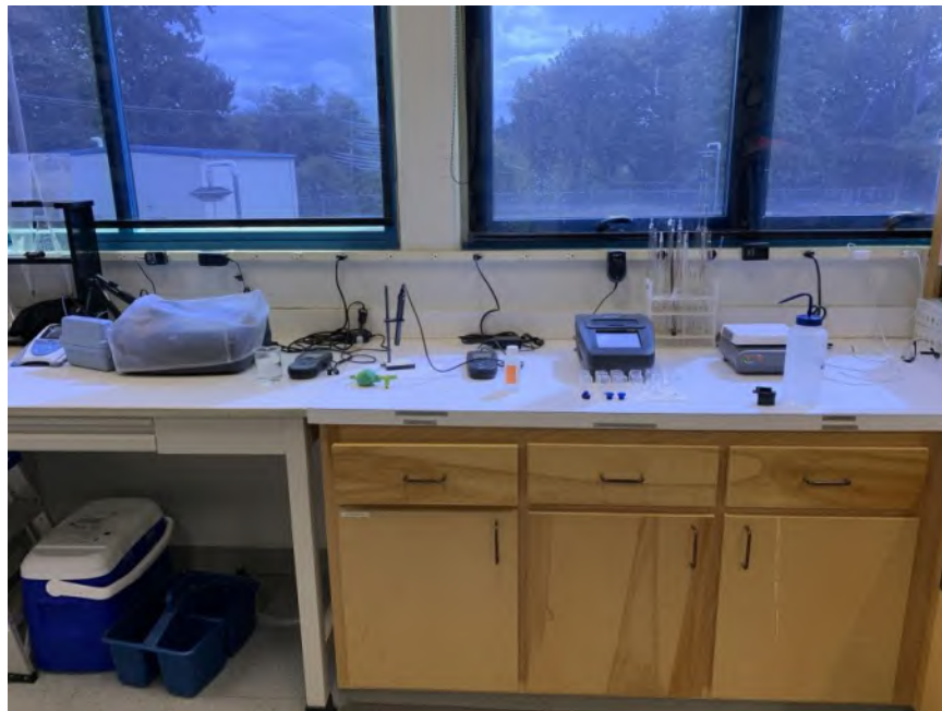
Figure 3.43 – Unrestrained Equipment on Lab Counter
