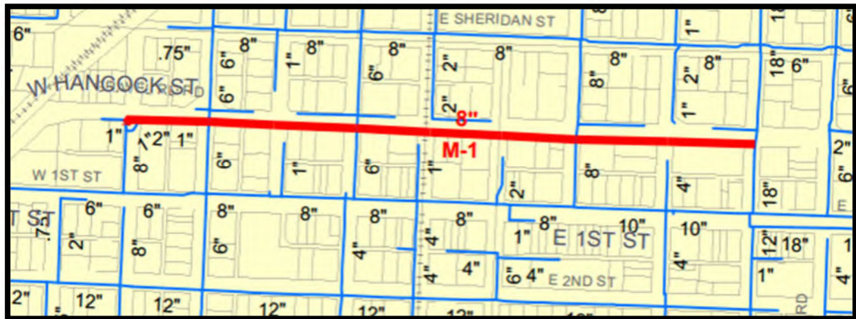
FIGURE 25 REPLACING DEFICIENT PIPE AND INADEQUATE FIRE HYDRANTS ON HANCOCK STREET
