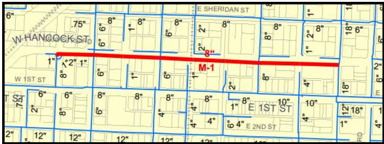
FIGURE 34 REPLACING DEFICIENT PIPE AND INADEQUATE FIRE HYDRANTS ON HANGCOCK STREET
