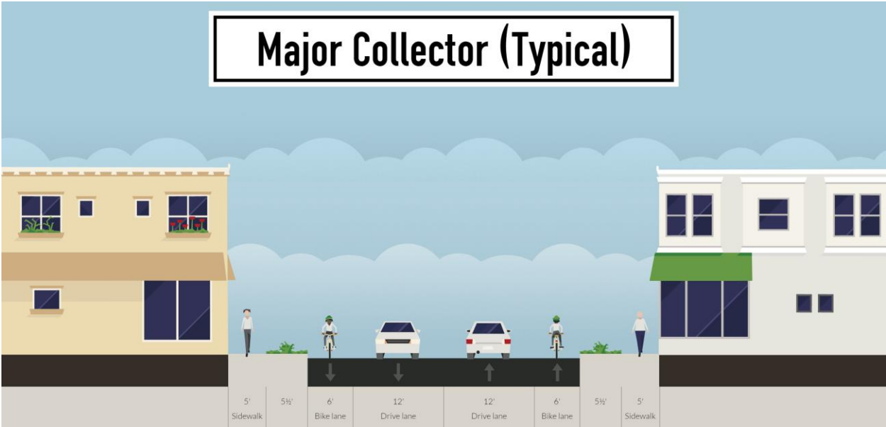
Figure 17: Typical Major Collector
