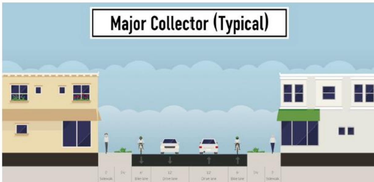
Figure 16. Typical Major Collector Diagram from Newberg TSP
