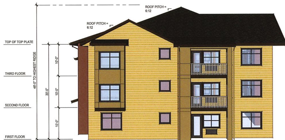
10. BUILDING TYPE A2 - TYPICAL END ELEVATION
