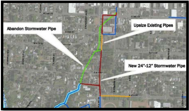
FIGURE 1 STORMWATER UTILITY LINES
