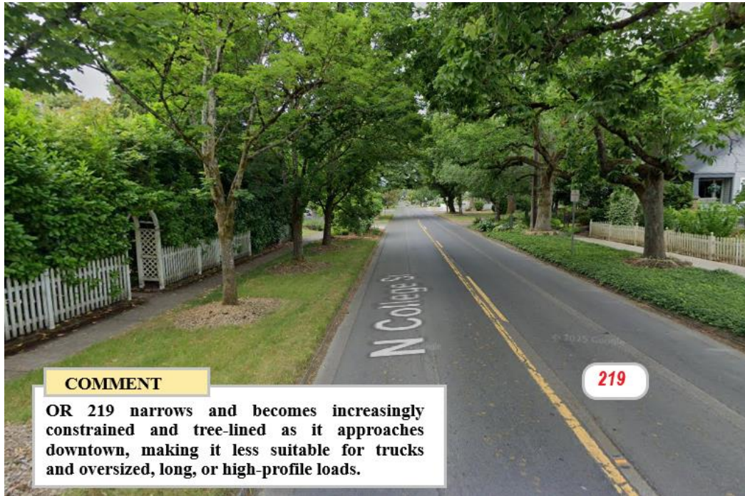
Figure 5 - As OR 219 approaches downtown Newberg, the roadway narrows and becomes increasingly constrained by mature street trees, on-street parking, residential development, and commercial activity. These characteristics reduce the corridor's suitability for frequent truck traffic, oversized vehicles, and other industrial movements when compared with the direct Major Collector connection provided by E. Illinois Street.
