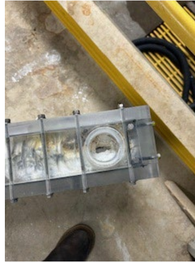
Generator Cell Blockage
